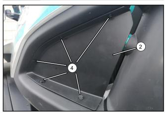
// Install the right door insert panel (2) in the right side door rear panel opening and secure it with plastic clips (4).
