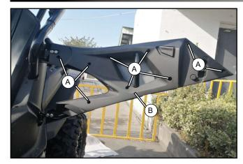
Remove screws (A) and passenger side inner door panel (B).
